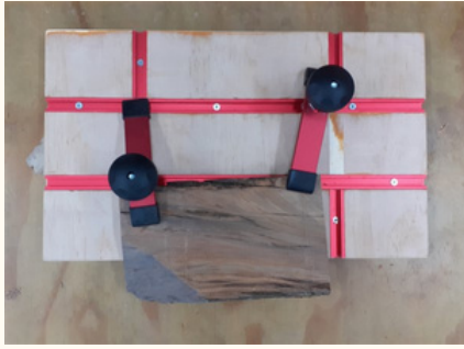
Mike's modified jig to cut a straight edge on the table saw
