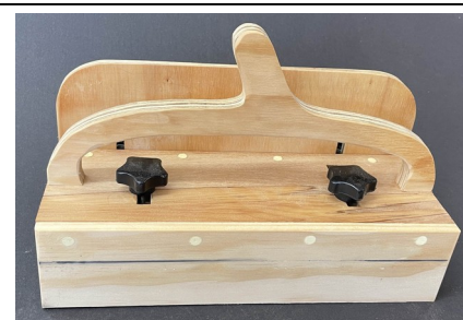
Duncan Campbell's jig to safely cut narrow strips on the tablesaw
