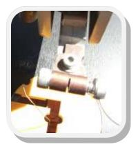
Method three; Roy Tregilgas made this one using part of a door hinge, knocking out the pin, and threaded the hole. After cutting the slot for the blade, he screwed a wing nut in one side, and a grub screw in the other side. A hole was drilled at right angles to fasten it to the machine. Instead of having a grub-screw you could have one screw from the side that is easy to get at, that goes right through the hinge with some lock-tight on one end, and when set cut your slot right through the screw.
