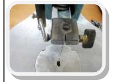
Method two; is what Jacob von Holzen made, and can be made the same way. Jacob cut the slot first and screwed a wing nut into one side, and a grub-screw into the other side.
