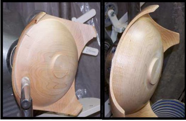
Photo #13: Ready to clean up the Edges Photo # 14 edges cleaned and bottom
