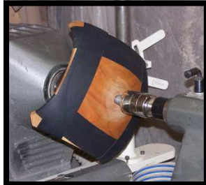
Photo #28: Lid taped in place
