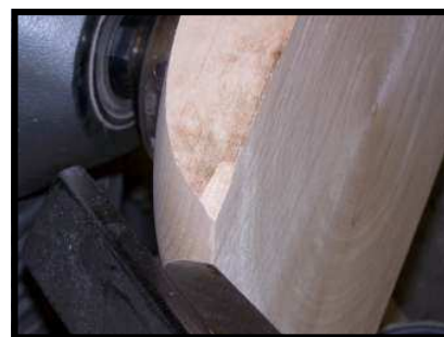
Photo #6: Corner sanded
