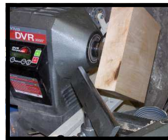
Photo#2: Face dressed and toolrest moved.
