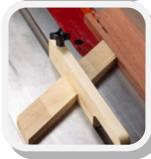
quards against dangerous kickback. To build one, use the drawing at right and patbandsaw to cut the 2 1/2"-long kerfs in the feather board and the curved portion of the handle, where located on the pattern. Cut the 30° angled notch in the handle's bottom edge using a dado blade in your tablesaw along with an auxiliary wood fence
