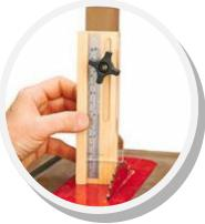
5/16" holes where shown and cutting out the material between them. Smooth the edges of the slot and the outer edges of the bar using a fine file. Buff the outer edges if you want to make them super smooth. Now, scribe a cursor line on the back face, where shown.
