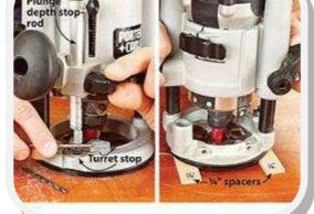
The method, at right, uses spacers planed to the same thickness as the depth of your plunge cuts. Place the router on a pair of spacers, and plunge the bit until it touches the benchtop. Then lower and tighten the stop-rod.
