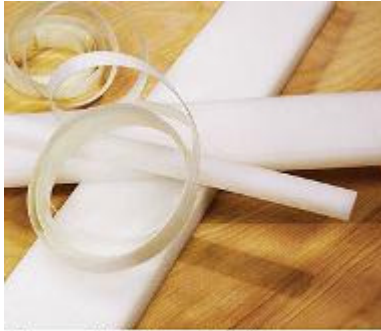
Slippery UHMW polyethylene comes as solid stock in many shapes and sizes or as self-adhesive tape. It's ideal for sliding jig bases or fence faces.
