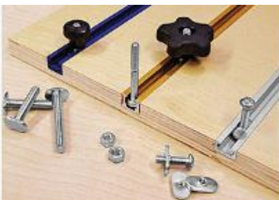
Use \frac{3}{8} "-deep T-track in thinner material. The track in the center accepts standard hex bolts and nuts. A 4' length of track costs less than $20.
