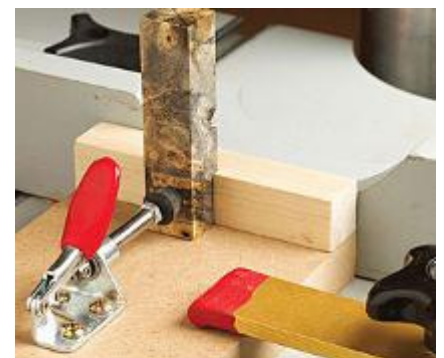
The horizontal toggle clamp on this jig safely and securely holds a small workpiece against a notched fence for drilling.
