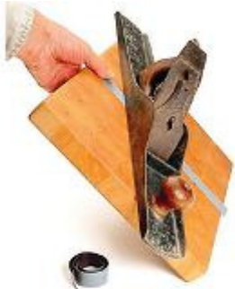
High-friction tape adds grip to a surface to prevent slipping without bonding or clamping. About $5 for 1x12", item 99K34.01, Lee Valley.
