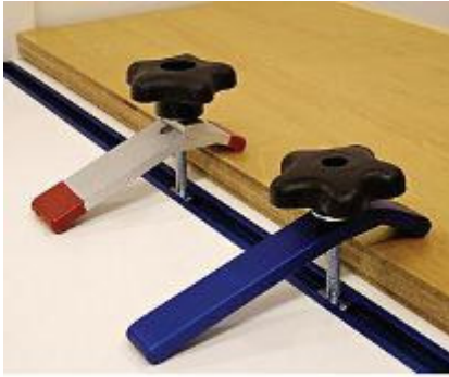
Hold-down clamps grip workpieces firmly. Increase capacity with a longer T-bolt and a block under the tail.
