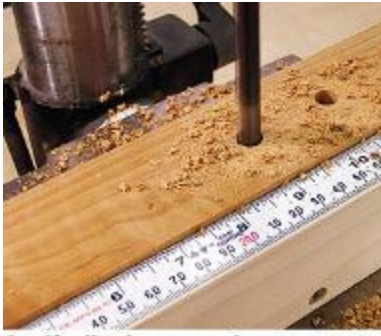
A self-adhesive measuring tape attached to a jig simplifies adjustment and work positioning. Tapes read left-to-right or right-to-left.
