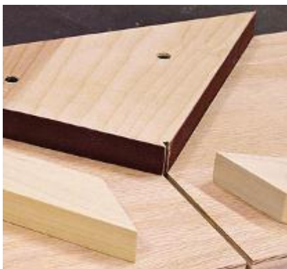
Self-adhesive sandpaper on this miter jig prevents slippage. About $17 for 2½"x30' roll, various grits, item 68Z72.01, Lee Valley.
