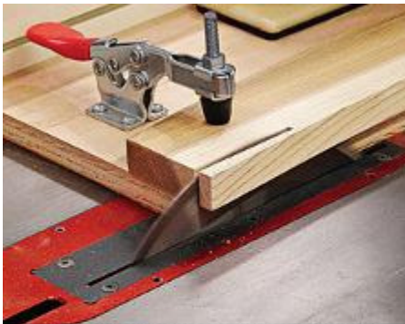
A vertical toggle clamp holds the workpiece firmly in place on this sled. The foot adjusts up or down to change tension or clamp thinner material.
