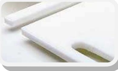
The nice thing about a plastic runner (like the one shown in the upper photo) is it won't swell or shrink with changes in humidity, so it will always slide smoothly without binding or slop. Plus, plastic is readily available. As you can see in the bottom photo, I simply cut a narrow strip from a plastic cutting board.
