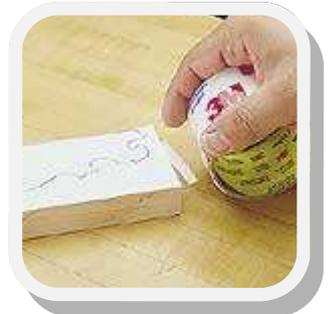
just cover the cutting line with a strip of cellophane tape, see left photo. (I use 2"-wide packing tape.)
