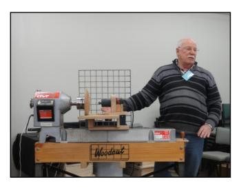
For the July group meeting, Roy Tregilgas demonstrated how he uses the indexing facility on a lathe to do decorative work, by using a trimming router which had been attached to his own home made wooden framework. This is another way to embellish your turned item.
