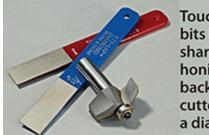
Touch-up router bits between sharpenings by honing the flat back of each cutter blade with a diamond file.
