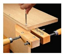
When installing woodscrews in the edge of manufactured materials like MDF, it's all too easy to split the sides of a workpiece — even if you drill a pilot hole first. To prevent this, I support the sides by clamping an ordinary hand-screw across the workpiece.
