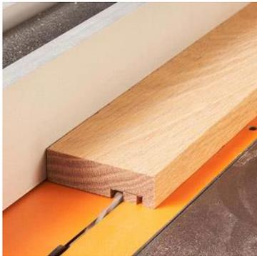
Every once in a while, a project plan calls for a quick groove or rabbet; but installing and fine-tuning the width of a dado set really kills your momentum in the shop. This simple method for cutting grooves and rabbets guarantees a perfect fit, even in odd-size plywood, using the blade already in your saw.
