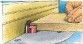
With a handheld router you typically use a rabbeting bit with a pilot bearing as shown above. You can change the width of the cut simply by changing bearings. And, with this setup you can even cut rabbets along curved edges.
