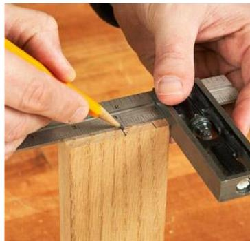
2. Now mark the location of the groove using a scribing knife or sharp pencil. Set the blade depth to match the depth of your groove -- no more than one-third the thickness of the stock.
