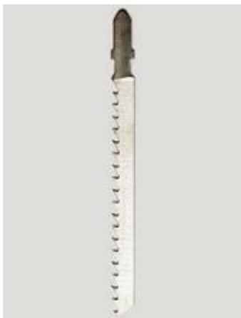
Standard 6-tpi blades use steep hook angles on the teeth and large gullets between them for quick waste removal. These blades work best when speed is more important than cut quality, such as working with construction lumber
