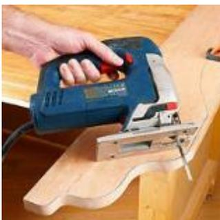
Choose the right tooth count for the cuts you make. Blades with aggressive 6-tooth-per-inch (tpi) designs work great for sawing construction lumber, but cut too coarsely for woodworking project parts. Instead, select a 10- to 12-tpi blade for larger, gradual curves, or a 20-tpi blade for tight curves (1" radius or less) in solid wood and all cuts in plywood or melamine-coated particleboard.
