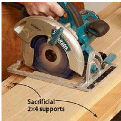
When crosscutting a board, place it on a pair of 2x4s. Then, with the blade set to cut slightly into the supports, cut your workpiece to length.
