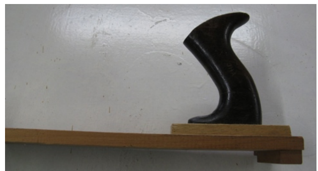
Buzzing a face SAFE The Bridge Guard can be placed so that a long piece long piece passes under it
