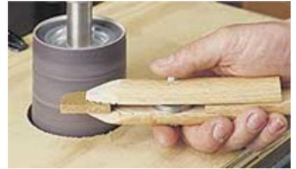
The jaws of the clamp are made from a short section of 1 1/4" dowel. The dowel is split down the centre and then the two halves are reassembled with a bolt, a wing nut and a few washers that space the "jaws" apart. A wedge inserted at the back of the clamp forces the jaws together.
