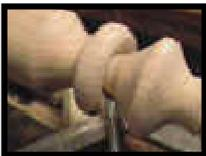
Continue working down each side with whatever tool you want. Here, I'm using just a small rounded skew.
