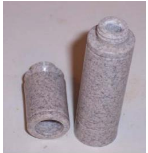
A needle case made from Corian. Corian threads very well. This one was not held with the disks, but only in the 25mm jaws of the chuck. I broke off the threaded tenon once and had to shorten the case.
