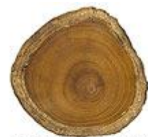
An off-center pith shows this tree's awkward growth. Irregular rings on a board's end are a subtle sign of growth stress.
