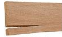
Splits appear in board ends where growth stress overcomes the interwoven wood fibers. The wood near the splits will likely warp further.
