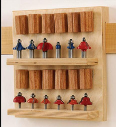
It often requires a second glance at a router bit to select the correct cutter for the desired shape. For a reference of the bit profile, rout an 8" length of scrap material with each bit. Crosscut the profile to a shorter length. With hook-and-loop material, hang the profile
