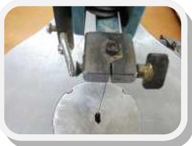
Method two; is what Jacob von Holzen made, and can be made the same way. Jacob cut the slot first and screwed a wing nut into one side, and a grub-screw into the other side.
