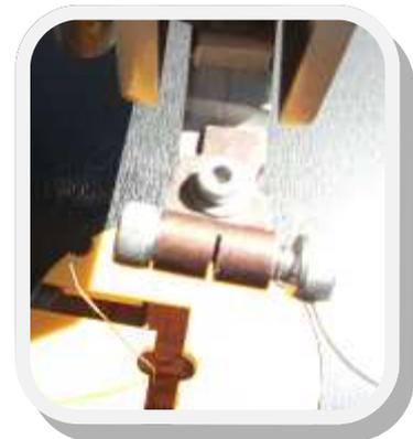
Method three; Roy Tregilgas made this one using part of a door hinge, knocking out the pin, and threaded the hole. After cutting the slot for the blade, he screwed a wing nut in one side, and a grub screw in the other side. A hole was drilled at right angles to fasten it to the machine. Instead of having a grub-screw you could have one screw from the side that is easy to get at, that goes right through the hinge with some lock-tight on one end, and when set cut your slot right through the screw.
