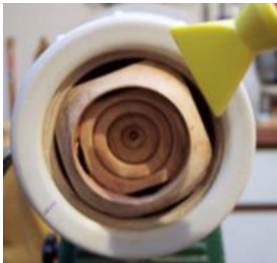
Picture 5. This photo shows that all of the first holes have been drilled and then the other levels on this hole have also been drilled.
