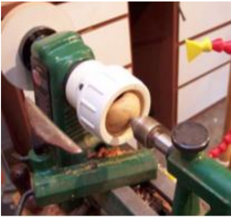
Picture 2. In this photo, the tail center is being used to align the ball on center before the chuck is tightened.
