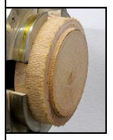
As you can see I cut a little too much off the jam chuck spigot, so I used a sheet of paper towel to get a tight fit. Finish the piece now. When the pieces are put together, they make an oyster shaped box, as shown in the next picture.
