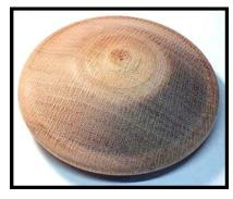
Turn a recess for the spigot to fit into. This
