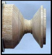
Next you will need to cut a radius on the edge and cut the back of the piece most of the way down. Try to maintain a constant thickness.
