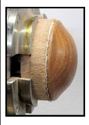
And here are the two halves, one with a bell and one with a spigot. The fit on these two mating halves is critical. Too tight and they won't go together. Too loose and they won't stay together. Be very careful with this.
