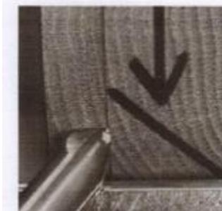
Note the arrow indicates the direction the wood is traveling past the tool. The 45-degree angled line shows the angle that will produce a clean slicing cut. To get this angle, twist the tool on its axis with your handle hand. The shaving comes off the right-hand side at the tip of the tool.
