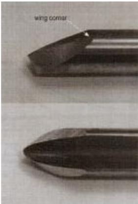
The side profile of Lyle Jamieson's favourite grind has nearly a straight line from the tip to the wing corner.
