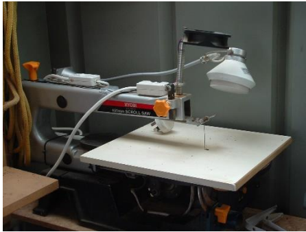
1. Ryobi scroll saw with pin less conversion
