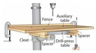
Super simple drill-press table Most of the auxiliary drill-press tables I've seen are unnecessarily complicated to install. This simple slide-on auxiliary table mounts to round or square drill-press tables, and you don't need to keep installing and removing bolts and nuts. Make the spacers about 1/16" narrower than the thickness of the drill-press table. Place the auxiliary table on the drill-press table before installing the cleats, and then tighten the
