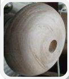
The wig stand head was turned first, with a flat base and an almost hemisphere top. This should measure about 140mm in diameter by 100mm high.
