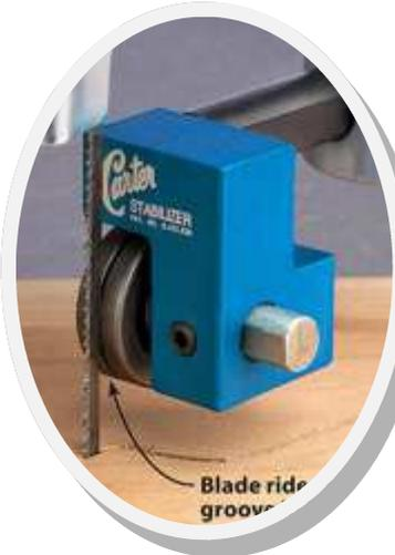
A specialized guide bearing helps narrow blades (1/8" and 1/16") track true during curved cuts. The rear of the blade rides in a groove in the bearing's edge. The groove provides side-to-side support and the bearing reduces friction.
