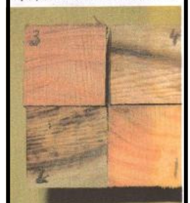
Photo.3 (above): The blocks are assembled in their final configuration and numbered. Photo.4 (below): They are then reassembled so that the outer faces face inwards
