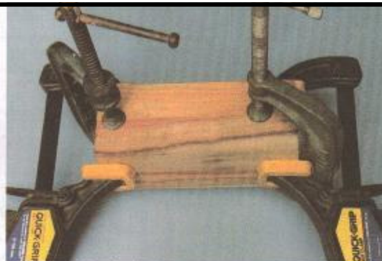
Photo.7: Gluing the four blocks — two sets of pairs — together
