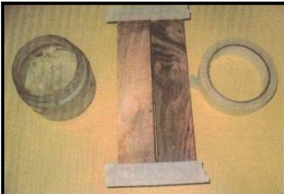
Photo.5: The blocks are first assembled in pairs. The wax (left) stops the glue from spreading into the centre of the blank
