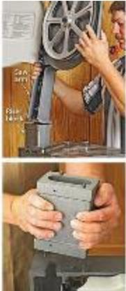
The typical riser block includes indexing holes on the bottom and matching pins on the top, so it's self-aligning. If your riser block has no pins, align the outer edges flush with the base. Reinstall the saw arm, as shown in the top photo.
