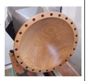
up and worked very well. Again, for safety sake, I used tailstock support; something that I do with any reverse turning method, whether it is a jam chuck, a vacuum chuck, a Longworth Chuck, or the Rim Chuck.
