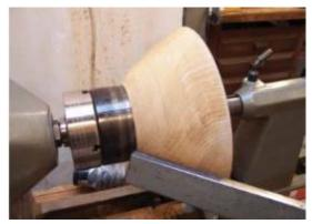
however, it fitted nicely into the Rim Chuck so I could turn the foot to fit my chuck (see the photo) below.
