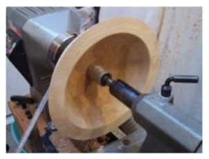
With the foot turned to fit into the chuck, I mounted the bowl in the chuck and final turned the outside and the inside. Incidentally, I used the cup-shaped live center to support the bowl in the Nova Chuck also. This allows more aggressive turning without concern of losing the bowl from the chuck.
