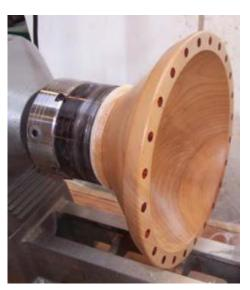
A view of the top of the bowl while still mounted on the lathe.
