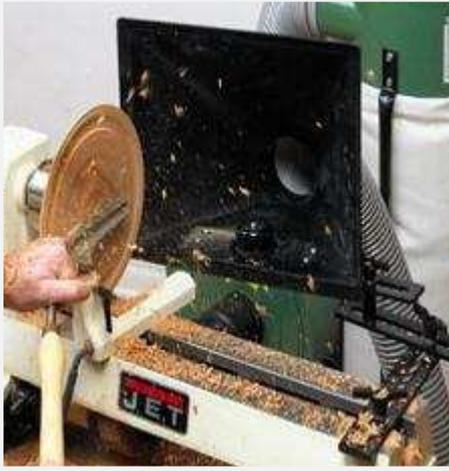
While no single accessory will catch all the dust and chips that go airborne when turning wood, the Big Gulp Ultimate Dust Hood gobbles up a lot of it. When tethered to a 1-hp or larger dust collector with 4" hose, the Big Gulp gathers in most of the chips made when hollowing out a bowl or vessel. It's especially effective at sucking up sanding dust from turnings--the stuff you'd breathe into your lungs otherwise.
