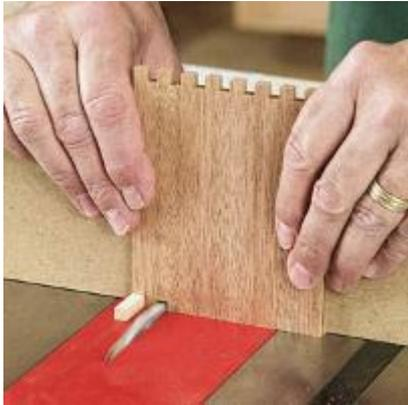
Waiting until the price is right to acquire a box-joint jig? By using shop scraps, we got the cost down to zero, and came up with a method that makes the box sides interchangeable for foolproof assembly
