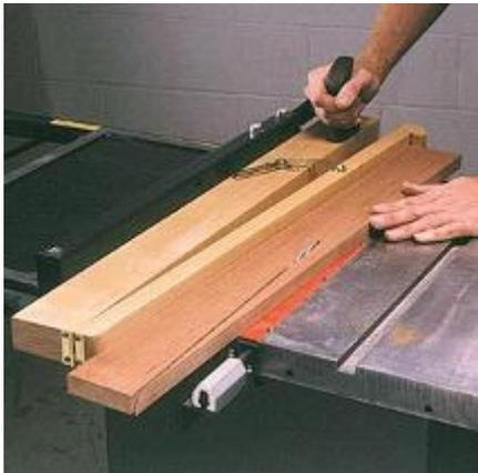
Ripping table legs or other project pieces at an angle can be frustrating and even dangerous work. However, with our taper jig, you'll be able to quickly set the precise angle and safely cut leg after leg, with the first identical to the last.
