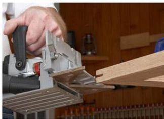
Here's how to do it. First, assemble your mitered project and allow the glue to dry. Cut two mirror-image triangles, as shown, mounting them to your joiner's fence with machine screws and nuts. Set your joiner's cutting depth as deep as you can. Trap the mitered corner in the fence jig and plunge a cut centered on the workpieces thickness. Then glue in the spline of your choice. When dry, trim it and sand flush.
