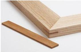
Splines add both strength and visual appeal to normally weak miter joints, especially when you make the spline from a contrasting wood species. Cutting the spline slots on your tablesaw requires a tall jig, but you can cut them easily and quickly with your biscuit joiner and the attached fence jig, see PDF file below.
