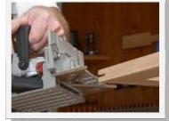
Here's how to do it. First, assemble your metered project and allow the glue to dry. Cut two mirror-image triangles, as shown, mounting them to your joiner's fence with machine screws and nuts. Set your joiner's cutting depth as deep as you can. Trap the mitred corner in the fence jig and plunge a cut centred on the workpieces thickness. Then glue in the spline of your choice. When dry, trim it and sand flush.
