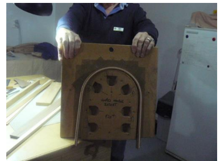
Photo 3 the former used to bend the wood
