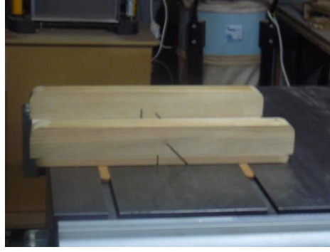
Photo 8 a sledge for the saw bench
