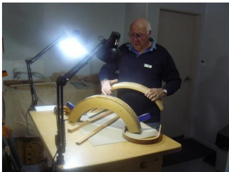
Photo 1 Mike with a bending former
