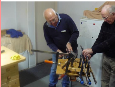
Photo 4 clamping the wood to the former
