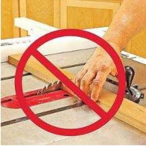
**Be alert!** The tablesaw-jury often begins with "I was making the last cut of the day..." Fatigue leads to errors in judgment that, in turn lead to miscut workpieces-or worse. Also, repetitive cutting chores can lull you to carelessness, so take frequent breaks.
