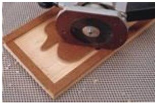
To make a recessed shape, use the arrangement shown below. If you want the shape to stand proud of the surface, go with the set-up shown in the photo at **left**. Once you're done routing, pop the template off the workpiece with a chisel.
