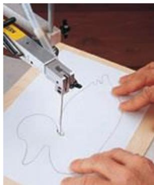
In most cases, 1/4" tempered hardboard makes the best choice for template material. It's inexpensive and easy to work with.
