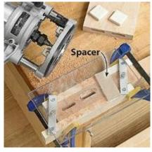
business. Install a 5/8" guide bushing in your router's subbase and a bit that matches the width of your mortise. Centre the scribed lines on the jig to your mortise layout lines, and then rout in 1/4"-deep increments. Depending on the position of your mortises, sometimes only one of the jig's aluminum cross bars will rest on the workpiece.
